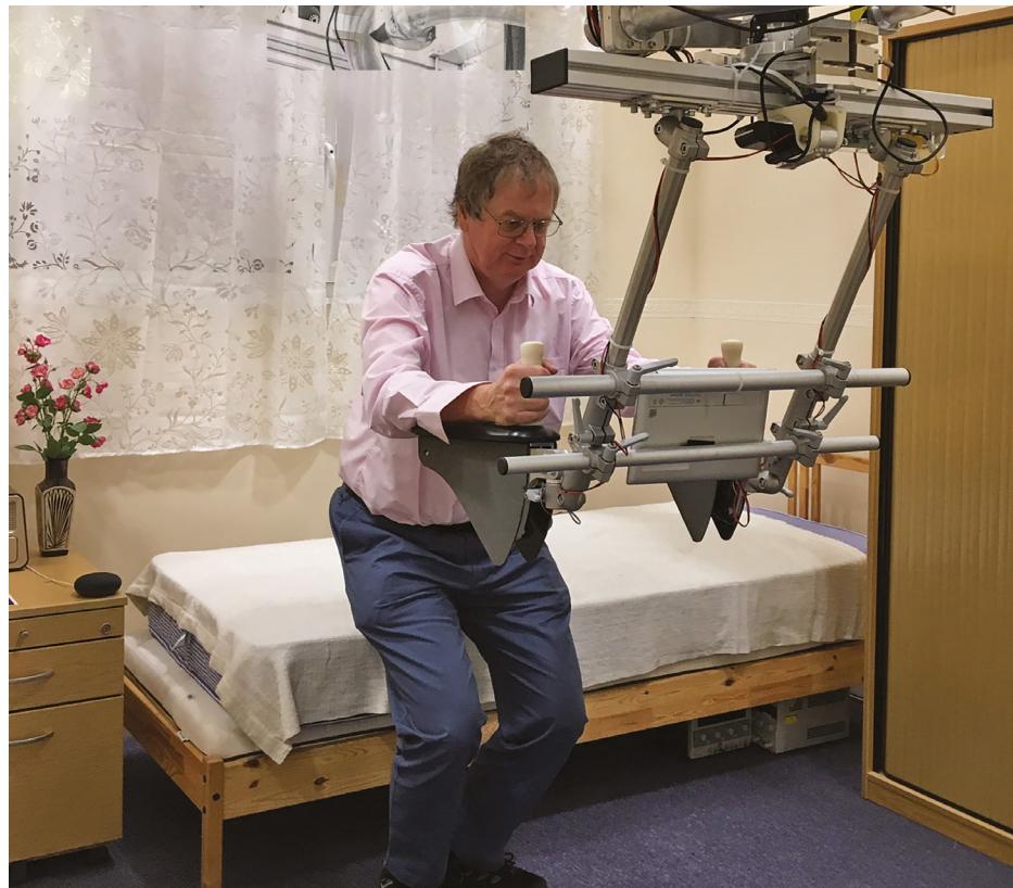
The sit-to-stand modular robot in the Bristol Robotics Laboratory assistive robotics test bed at UWE
